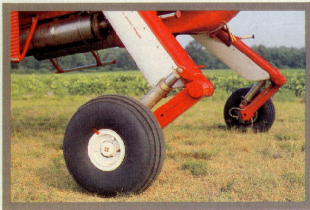
Fixed slats on the leading edge improve low-speed handling and short field performance. Stumps and rocks pose no problems for the hefty gear struts.
